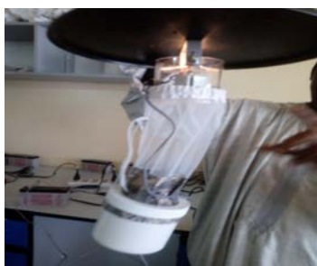
Fig. 39: Setting up of CDC Light Trap
